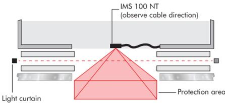
Figure 2: Mounting position - center opening door
