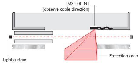
Figure 4: Mounting position - left side-opening door
