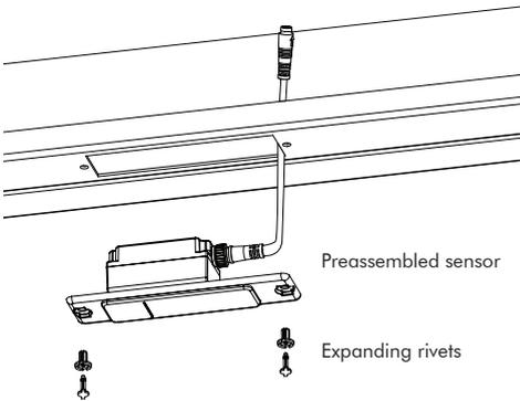
**Figure 8:** Flush mounting (center opening doors)
