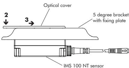
Figure 24: Optical cover - press (2) and slide (3)
