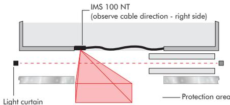
Figure 3: Mounting position - right side-opening door
